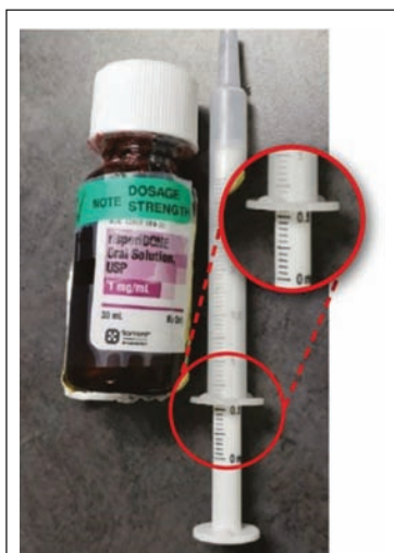
Figure 2. The dosing devices packaged with risperiDONE oral solutions may contribute to dosing errors because the measurement graduations are on the plunger unlike most oral syringes that have the graduations on the syringe barrel.
